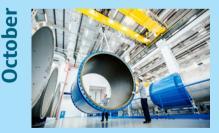
Endress+Hauser celebrates the manufacture of its 3-millionth **electromagnetic flowmeter** since 1977. With these instruments, customers can reliably measure the volume flow of conductive liquids in pipes with diameters ranging from a tiny 2 millimeters to a massive 3 meters.
